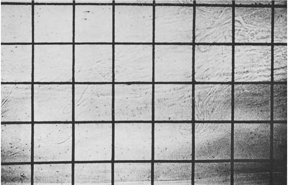
FIGURE 8. Wave breaking and roller formation at low values of Ri^* ( \approx 2 ). The density inflexion point is about 3 cm from the bottom of the picture. Note the eddies from breaking waves which have penetrated into the region of maximum density gradient and the disturbances along the top of this region. Background grid is 2 cm by 2 cm.
